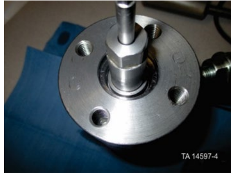
Place the tool on the jam nut
