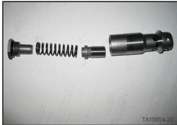
Relief Valve Assembly Inspection
