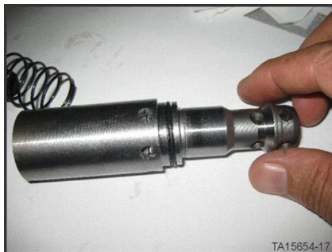
Anti-Void Spool Assembly removal
