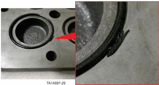
Seal Inspection (Damaged seal shown for example purposes)
