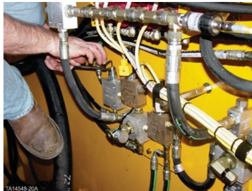
Secondary dump pressure relief 800 psi (55 bar) SOL SD
