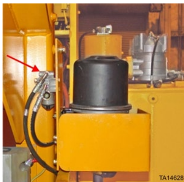
Location of compressor governor
