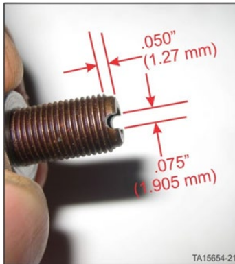
Adjustment Screw Groove dimensions
