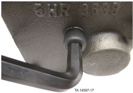
Steering Amplifier End Cap removal socket head capscrew (picture shows 2 of the 8 bolts previously removed)
