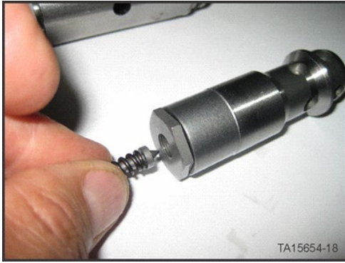
Relief Valve Cone and Spring removal
