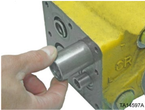
Installing the Shock and Suction Valve into the Steering Amplifier body (CR Port End shown)
