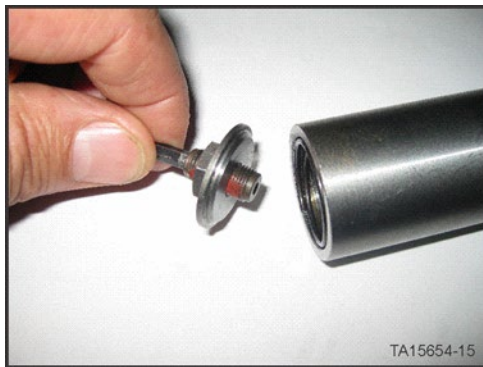
Relief Valve Adjustment Screw installation
