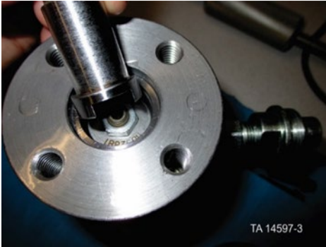
Align the flats to the jam nut
