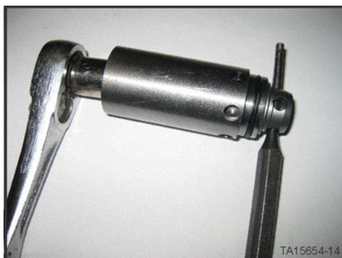
Loosening of the adjustment screw jam nut
