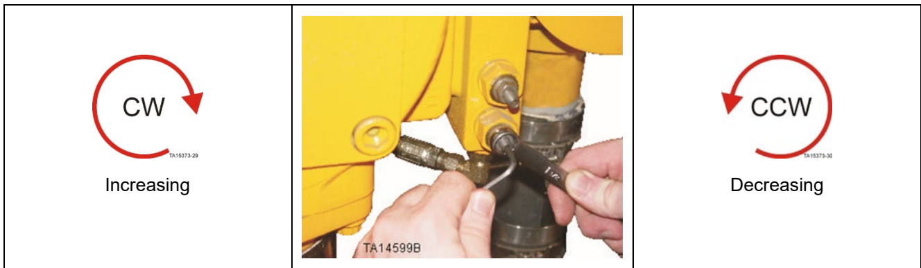
Figure 8. Fan standby (flow) compensator
