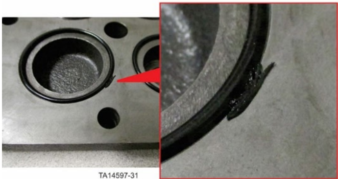
Example of a damaged O-ring
